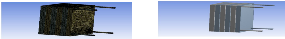
Fig 4. Mesh model and CAD model of plate type heat exchanger
